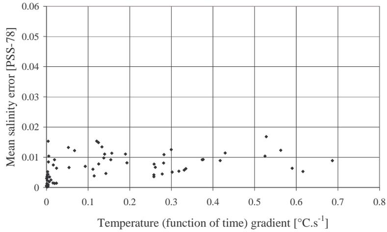
FIG. 5. Same as Fig. 4 but with the new parameters. The maximum salinity error is 0.017 against 0.050 in Fig. 4.
