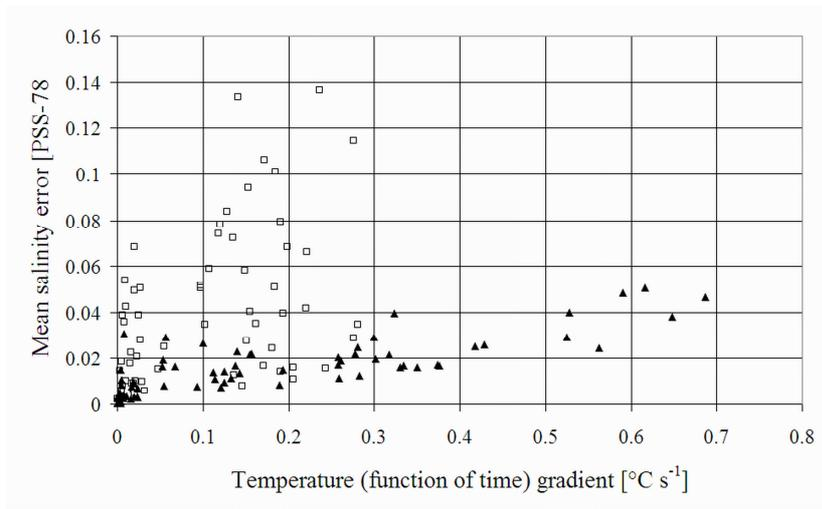
FIG. 2. Mean salinity errors calculated with PSS-78 formulas, as a function of the temperature gradient. Empty squares represent the profiles with strong salinity gradients (superior to  $0.01 \text{ s}^{-1}$ ), plain triangle shows profiles with weak salinity gradients (less than  $0.01 \text{ s}^{-1}$ ).
