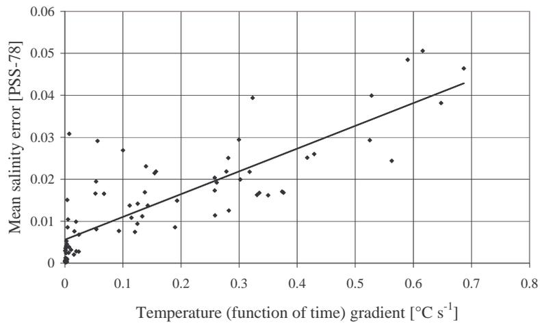
FIG. 4. Salinity error as a function of temperature gradient, for standard parameters (zoom of Fig.2, retaining only profiles with weak salinity gradients).
