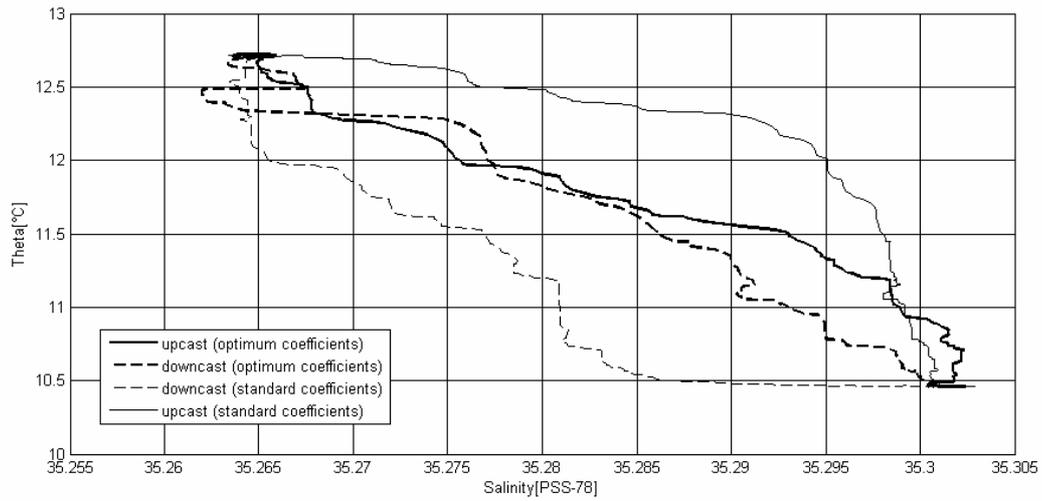
FIG. 3. Theta-S plot of a profile with strong temperature gradient (see Fig 1b). Thick lines represent the results with optimal coefficients, while thin lines show the results for standard coefficients.
