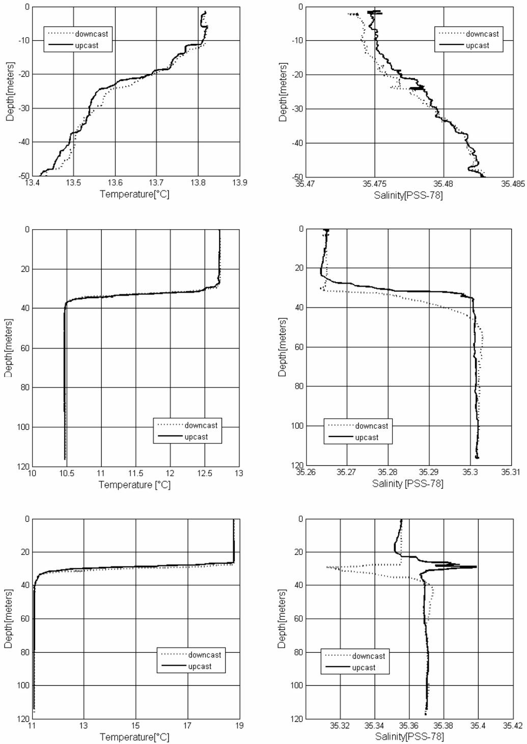
FIG. 1. Temperature and salinity upcast and downcast profiles for 3 different temperature gradient conditions. (a) Weak ( $0.01 \text{ } ^\circ\text{C s}^{-1}$ ) temperature gradient. (b) Strong ( $0.2 \text{ } ^\circ\text{C s}^{-1}$ ). (c) Extreme ( $0.7 \text{ } ^\circ\text{C s}^{-1}$ ).
